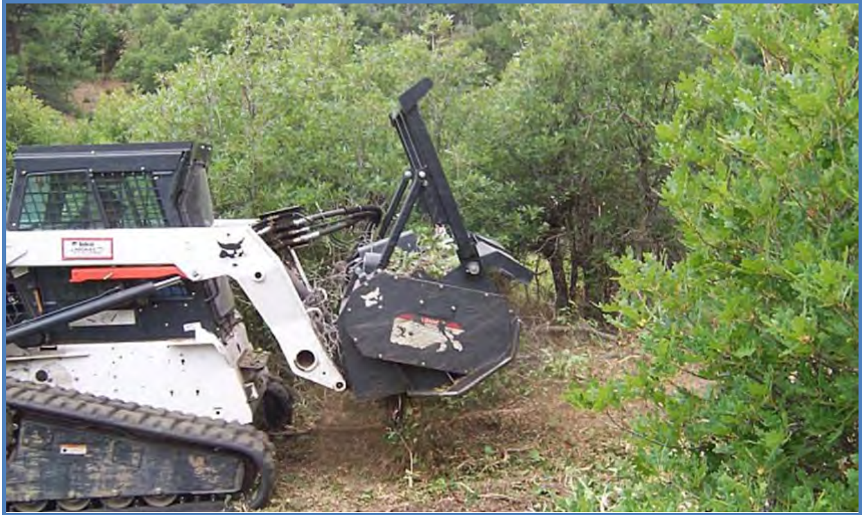
Figure 26. A Skid Steer with a masticating head shredding Gambel oak for one of the demonstration projects. The machine leaves shredded oak on the forest floor that breaks down and becomes nearly unnoticeable in a couple of years.
